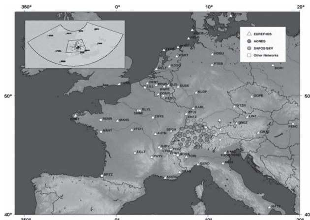
Figure 1. The Swiss Permanent Network AGNES nested in the networks of EPN and IGS.
