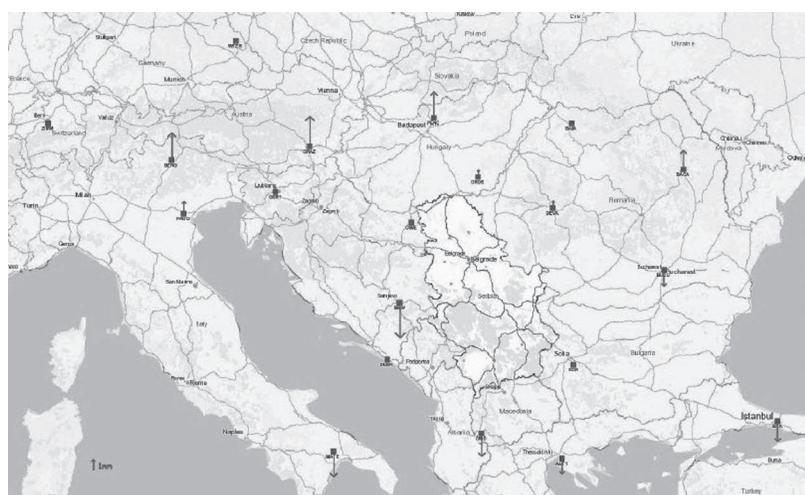
Figure 4: Differences of reference EPN stations height
