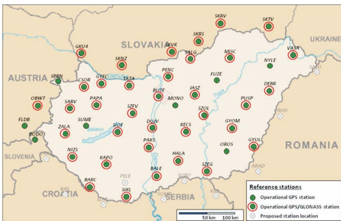
**Figure 1.** The GNSSnet.hu reference station network
