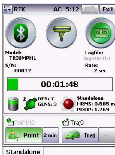
Figure 2-6. Point surveying in progress
