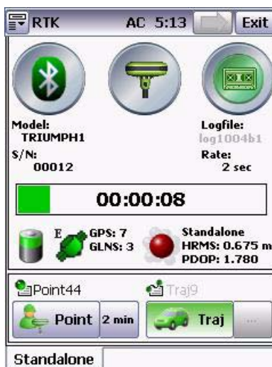
Figure 2-7. Trajectory surveying in progress
